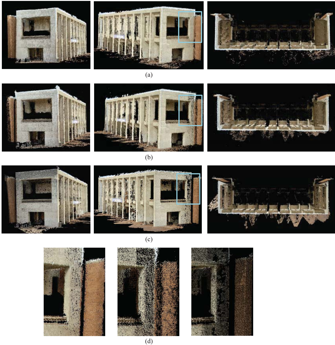
Fig. 15. Final reconstruction results (colorized point cloud rendering) of three evaluated methods on the Hull data set. In (a)–(c), the results are rendered from three different view points (the right one is seen from the top view).
